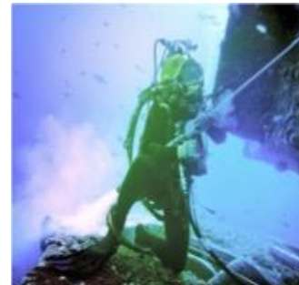
Hull cleaning by divers for UWILD
