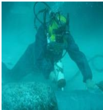
Diver measuring corrosion protection level of pipeline
